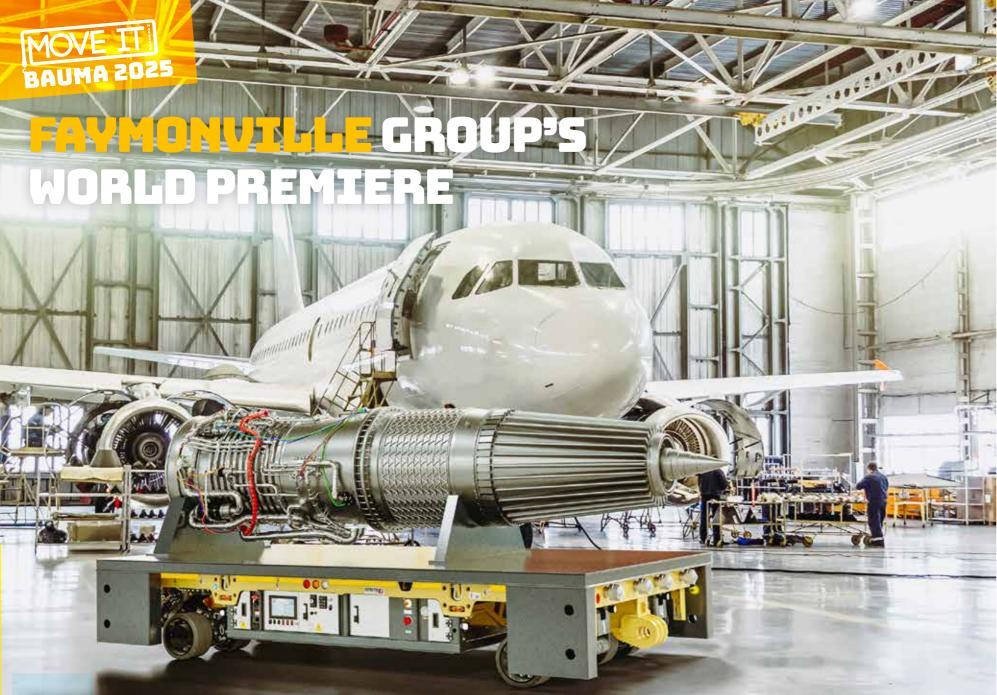
150 tons are possible-depending on local regulations for axle and kingpin loads or in off-road conditions. These are unique capacities for a vehicle whose loading platform extends from 20 meters to an impressive 41.9 meters in just minuteswhile maintaining full payload capacity!
