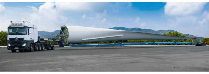
ooteboom Trailers is introducing the innovative Super Wing Carrier XL (SWC-XL), setting a new standard in wind turbine transport. Specially designed to transport the latest wind turbine rotor blades exceeding 85 meters in length, this cutting-edge trailer offers unmatched stability, safety, and flexibility for the growing demands of wind turbine logistics.
