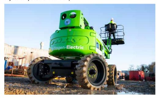
machine, the hydrogen fuel cell system does add a small amount of extra maintenance, but this is generally less intensive than diesel engine maintenance and is offset by increased uptime and reduced downtime for charging.
